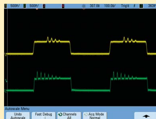
Figure 3: A DDS generator (upper trace) was unable to output all seven aberrations in this 2 MHz arbitrary waveform.
