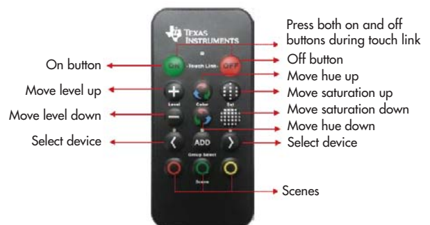
2. The ZLL Remote Control can manage an array of ZigBee-based lights.
