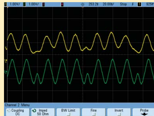
Figure 1: Signals at the same frequency created by a DDS generator (upper trace) and a Trueform generator (lower trace)
