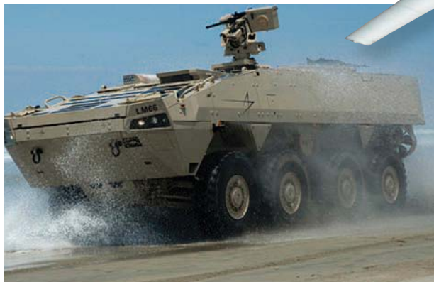
1. Havoc is a UGV with an 8x8 drive system that can conquer a wide range of rough surfaces. [Photo courtesy of Lockheed Martin ( www.lockheedmartin.com )]
