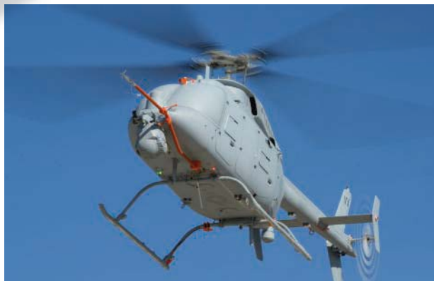
2. The MQ-HC Fire Scout is an unmanned helicopter capable of capturing real-time video information. [Photo courtesy of Northrop Grumman ( www.northropgrumman.com )]
