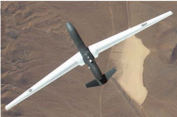
4. BAMS-D UAVs were modeled on the Global Hawk UAV but designed for maritime use. [Photo courtesy of Northrop Grumman ( www.northropgrumman.com )]
