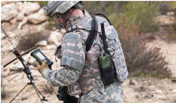
2. The AN/PRC-152A is truly a multiband radio, with total frequency range extending from sections of 30 to 870 MHz. [Photo courtesy of Harris Corp. ( www.harris.com )]
